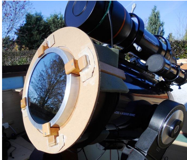
Figure 2 – An 8" Thousand Oaks White Light Filter
