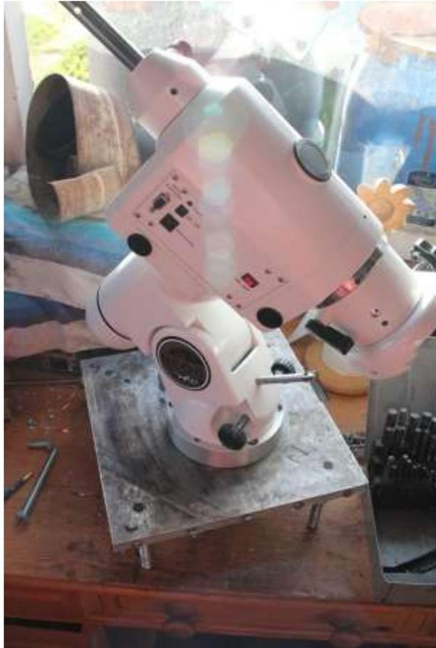
**Figure 7 - Offering up the EQ6 to the pier adaptor**
