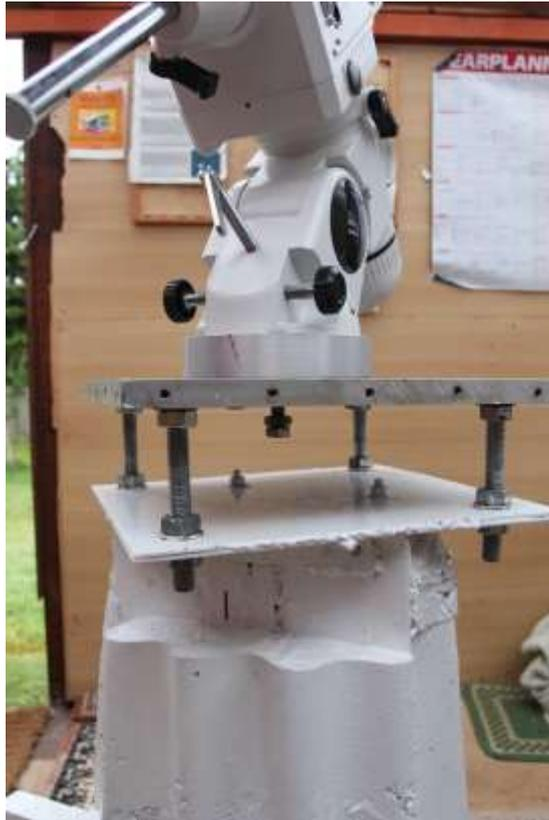
**Figure 11 - Tighten the EQ6 central bolt**
