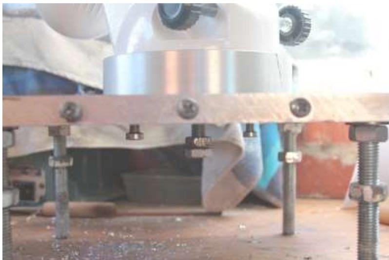
**Figure 8 – Check that the central bolt engages with the EQ6**
