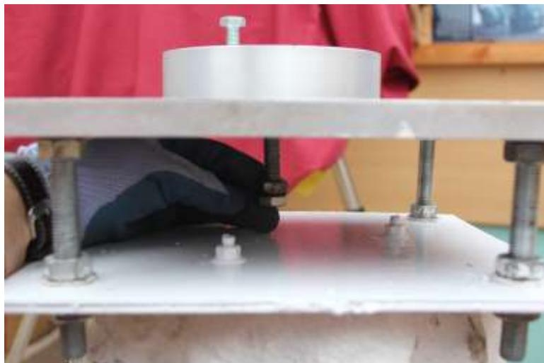
**Figure 10 – Get ready to bolt the EQ6 in place**
