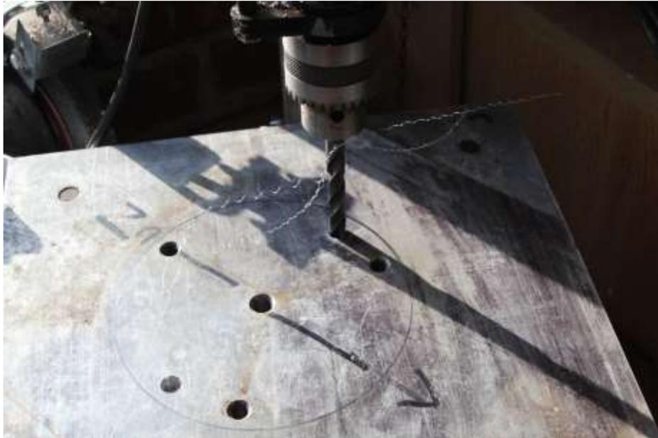
**Figure 5 – Drill 4 holes for bolting the adaptor to the top plate**
