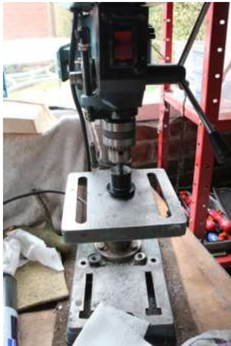
Figure 7 – Skimming the T adaptor bore
