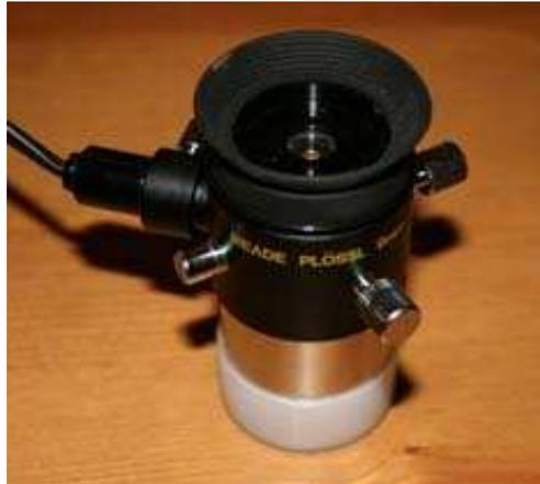
**Fig. 1 – An illuminated Guiding Eyepiece (9mm) with cross-hair adjustment**
