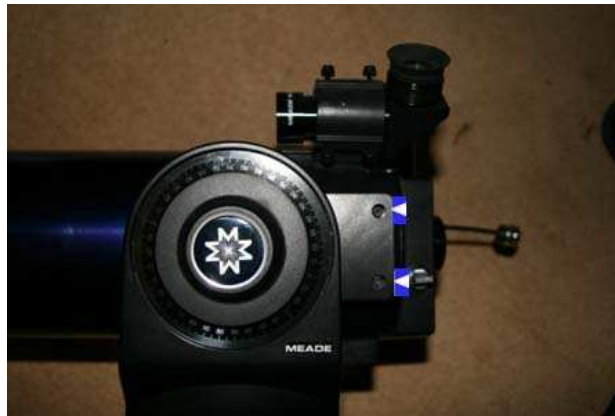
Fig. 1 – OTA Retention screws arrowed
