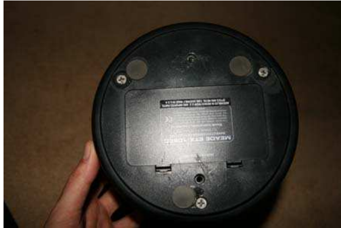
Fig. 10 – Reveal the three base screws
