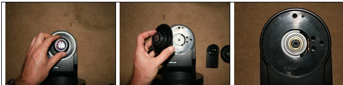
Fig. 9 – Declination scale removal – Second Arm
