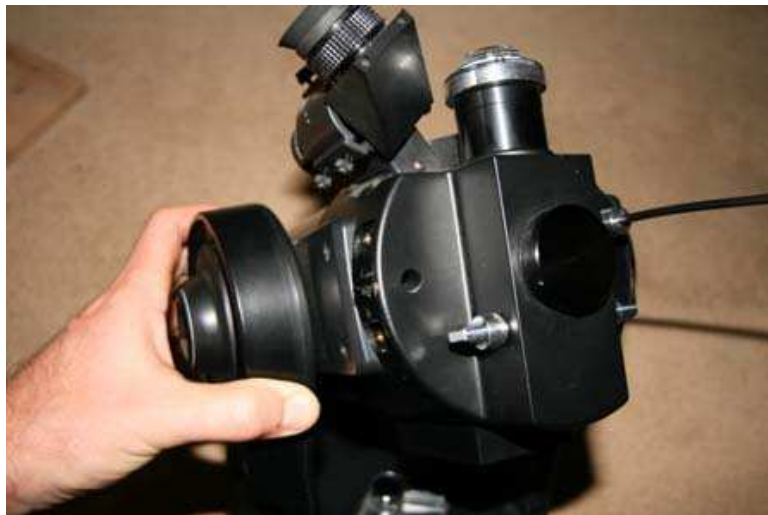
Fig. 4 – One arm raised up to clear the OTA
