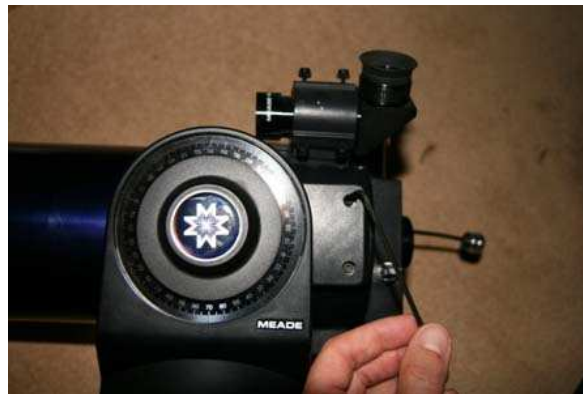
Fig. 2 – Removal of OTA retention screws
