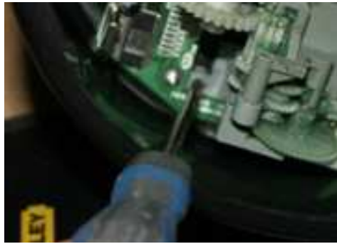
Fig. 14 – Remove the three screws holding down the circuit board and gear assembly
