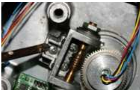
Fig. 13 – Remove the three screws holding down the worm
