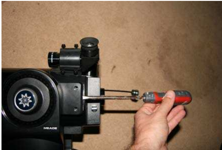
Fig. 3 – Raising up one arm to release the lugs
