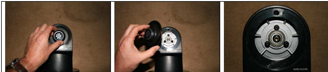
Fig. 8 – Declination scale removal – First Arm
